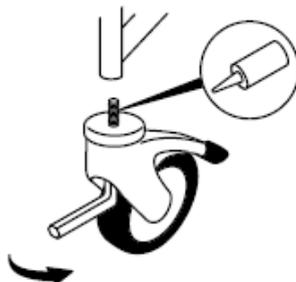
**NB: Where leg extension pins are in place it is recommended that the extension pins are replaced at the same time as the castor.**
